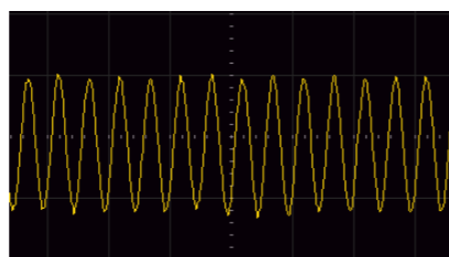
20mVpp signal measured by 12-bit XDS series DSO, 10 times zoomed
